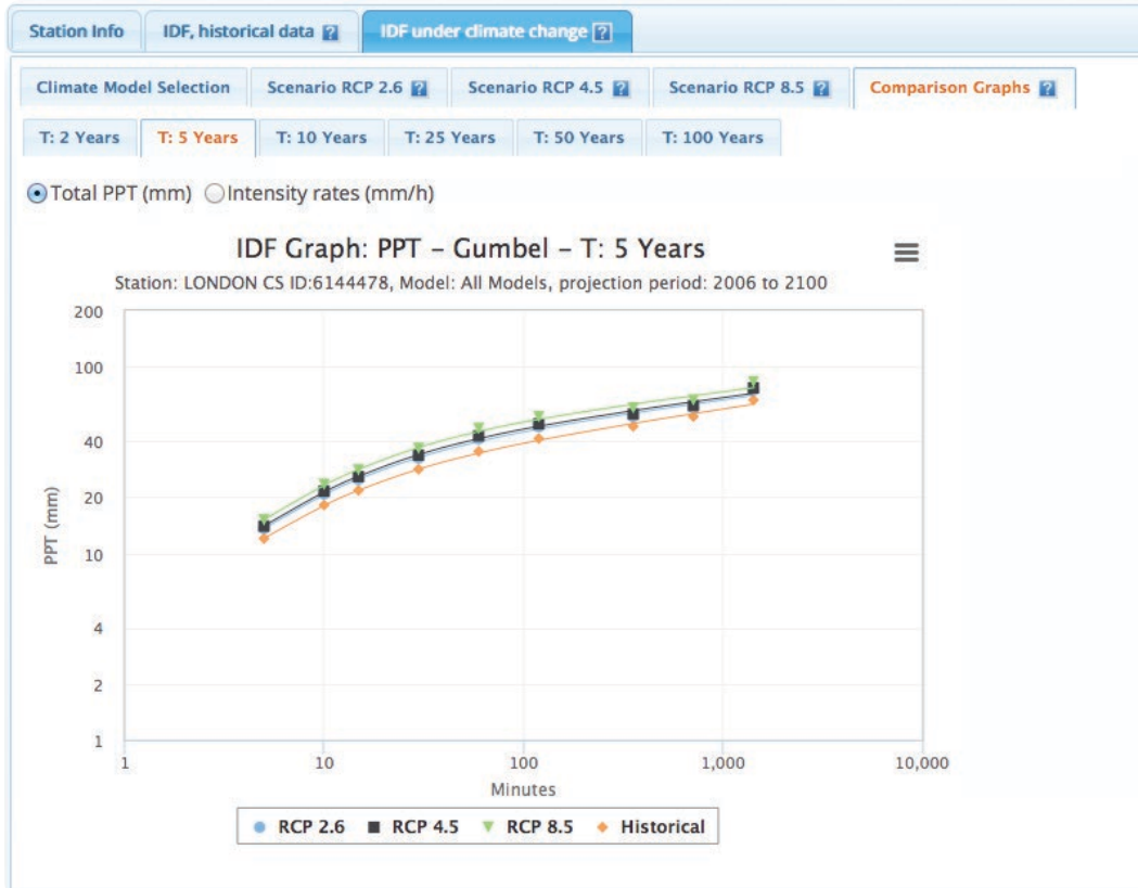
Figure 4: Sample IDFCC Tool output - An IDF curve updated using the ensemble option and RCP 8.5. Users can compare historical IDF curves to curves that incorporate GCM outputs. Users can also click different tabs to compare outputs for different RCPs and rainfall return periods.
