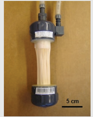
Figure 2. Image of the small-scale membrane modules used during laboratory studies as part of this research.
