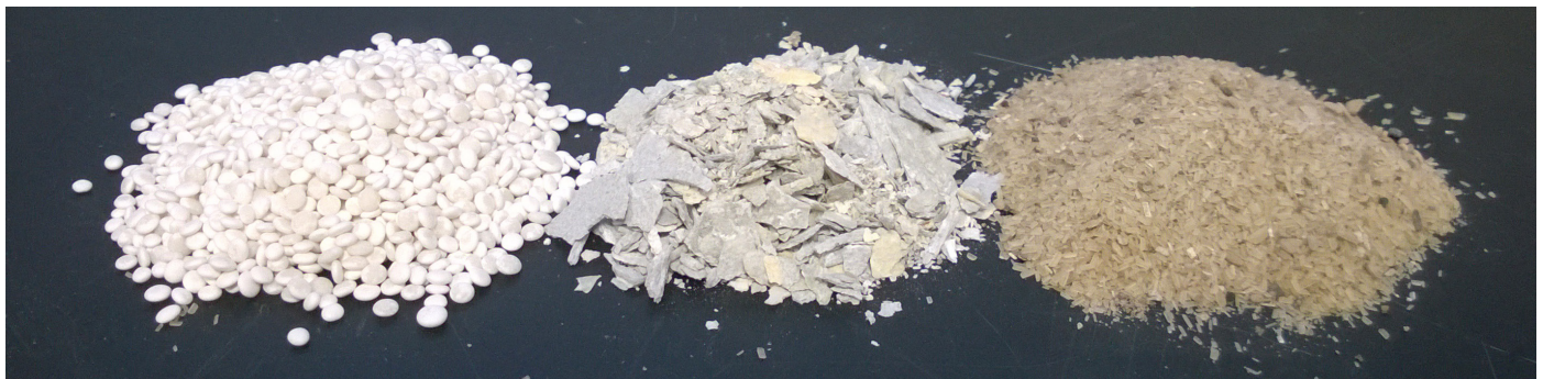
Figure 6. Various form of recovered struvite. From left: Ostara Pearl, electrochemical method, AirPrex. Photo: D. Kruk, University of Manitoba
